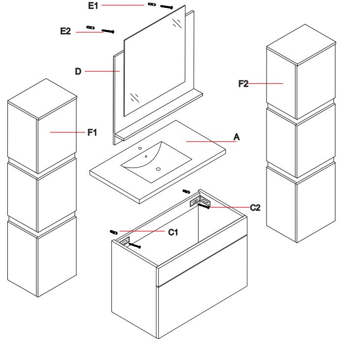
1. Install the cabinet on the wall using the screws (C1,C2) as below Picture.
