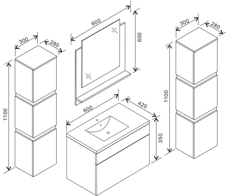
3. Measure the distance of the mirror's back brackets, and install the screws on the wall, then hang the mirrors on the screws.
