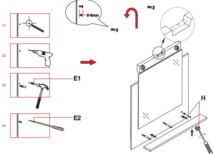
4. Install the side cabinet according to the diagram below
